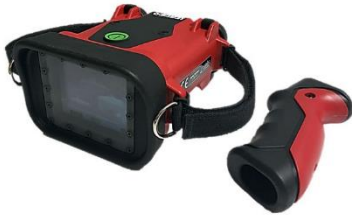
LEADER TIC 3.1 with 1 button (detachable optional pistol grip)
